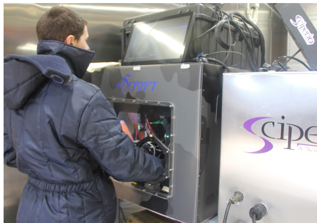
A representative from nScript demonstrates its Austere nField Repair, a rugged "factory in a box" that employs additive electronics and mechanical part manufacturing to replace and repair damaged hardware, during the OSD ManTech Program's Point of Need Challenge held at the U.S. Army Engineer Research and Development Center's Cold Regions Research and Engineering Laboratory in Hanover, New Hampshire, December 7, 2023
